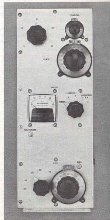
PANEL VIEW of the linear amplifier. Note that grid and plate bandswitches have separate knobs, and are not ganged. Snap-in buttons cover the holes through which the neutralizing capacitor ( C_1 ) and bias potentiometer are adjusted.
